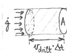
$$\Delta V = A \cdot v_{drift} \cdot \Delta t$$
