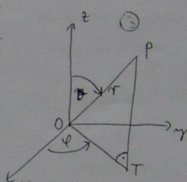
$$\left. \begin{array}{l} x = r \cos \theta \sin \varphi \\ y = r \sin \theta \sin \varphi \\ z = r \cos \varphi \end{array} \right\} \quad \begin{array}{l} \theta \in [0, \pi] \\ \varphi \in [0, 2\pi] \\ r \in [0, \infty) \end{array} \quad \textcircled{3}$$
