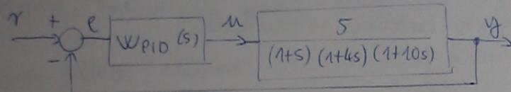
$$W_o(s) = \frac{A_p}{T_F} \cdot \frac{s^2 T_I (T_D + T_C) + s (T_I + T_C) + 1}{s (1 + T_C s)} \cdot \underbrace{\frac{5}{(1+s)(1+4s)(1+10s)}}_{40s^2 + 14s + 1}$$
