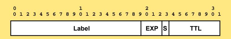
Label = 20 Bits COS/EXP = Class of Service, 3 Bits S = Bottom of Stack, 1 Bit TTL = Time to Live, 8 Bits
