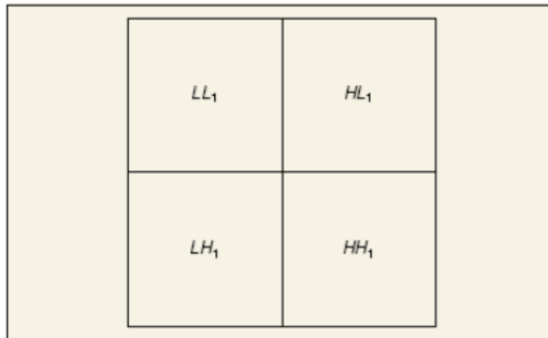
▲ 4. The subband labeling scheme for a one-level, 2-D wavelet transform.
