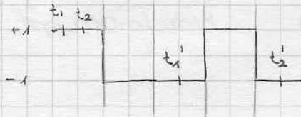
$$P_{X_1, X_2}(x(t_1), x(t_2)) = \begin{cases} \frac{1}{2} [\delta(x_1-1)\delta(x_2-1)] + \frac{1}{2} (\delta(x_1+1)\delta(x_2+1)) \\ \quad t_1, t_2 \text{ e.v. ozonos} \\ \frac{1}{4} \delta(x_1-1)\delta(x_2-1) + \frac{1}{4} \delta(x_1-1)\delta(x_2+1) + \frac{1}{4} \delta(x_1+1)\delta(x_2-1) + \\ \quad + \frac{1}{4} \delta(x_1+1)\delta(x_2+1) \end{cases}$$
