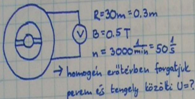
$$U = \frac{R^2 \omega B}{2} = \frac{R^2 2\pi n B}{2} = \underline{\underline{7.07\text{V}}}$$
